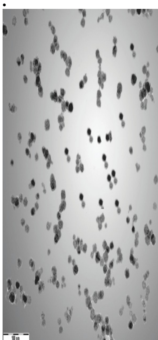
Fig. 9. TEM micrograph of silver nanoparticles synthesized by Penicillium fellutanum . [39]
