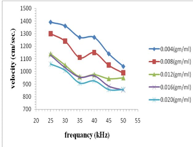
Fig(1) Ultrasonic velocity due to frequency
