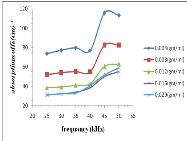
Fig(7)absorption coeffi. due frequency
