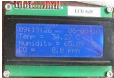
Figure.13. LCD screen display monitor when the humidity reaches a maximum value
