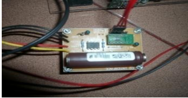
Figure-5. Circuit of SHT11
