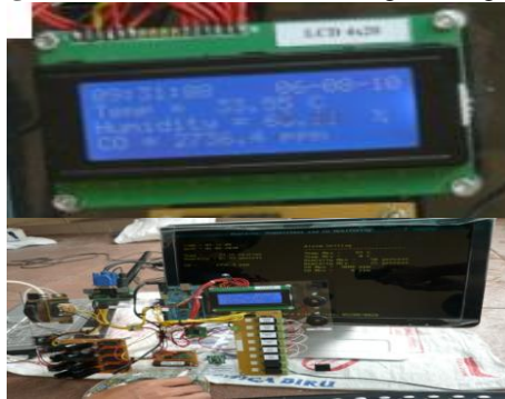
Figure-7. The sensor detects CO gas of cigarette
