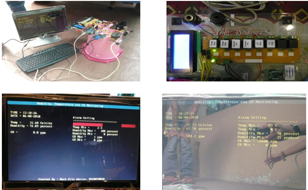
Figure-9. Sensor detect CO gas from the car with biodiesel fuel
