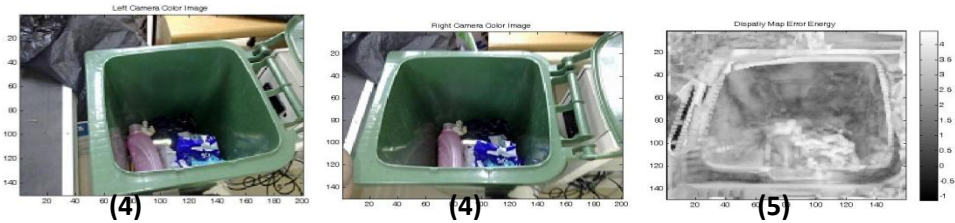
Figure- 4. True Colour Test images: Right and Left Images; FIGURE 5: Error Energy Minimization for point matching window (1x1)
