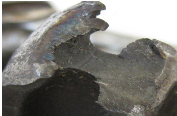
Fig-4. Fractured surface at the end of connecting rod
