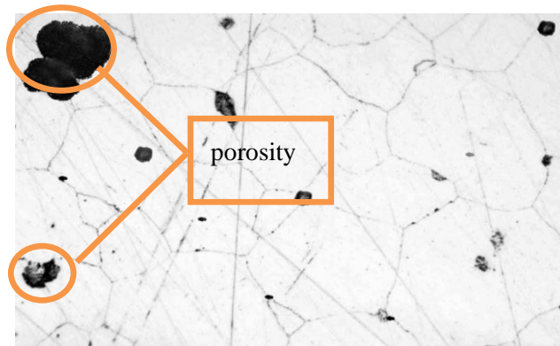
Fig-5. Metallographic of casting defect of the connecting rod
