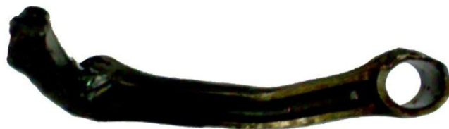
Fig-1. Failure on Connecting Rod
