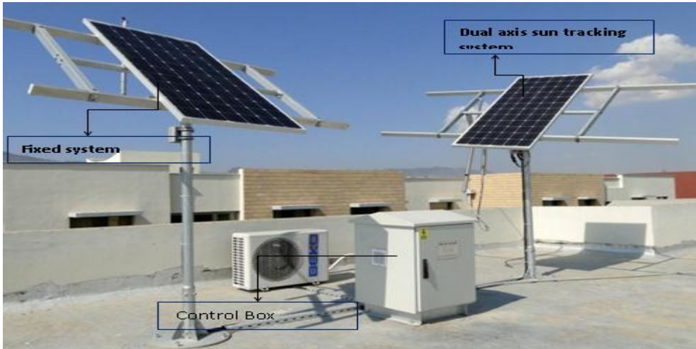
Figure-3. Experimental set-up of the fixed and dual axis sun tracking system
