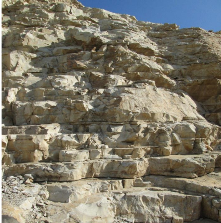
Fig-2. A section of limestone's beds in Chaqchaq Quarry showing the different thickness ranging between 5-80 cm.
