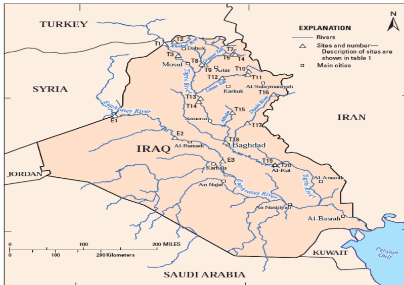
Figure-2. Locations of stream flow gauging stations for Tigris River and Euphrates River Basins, Iraq.
