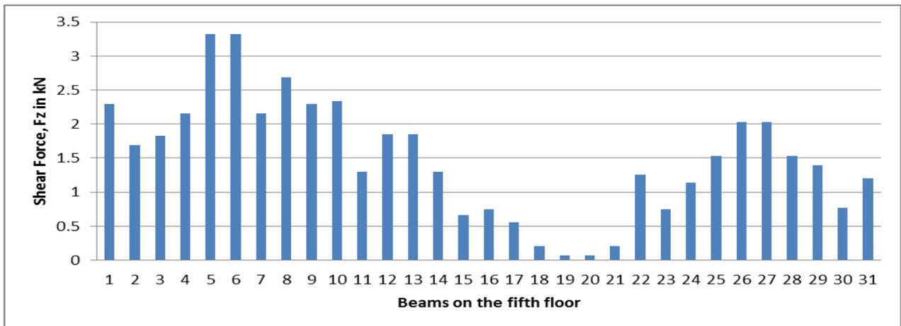
Graph-No. 9. Shear Force (Fz) for the beams on fifth floor
