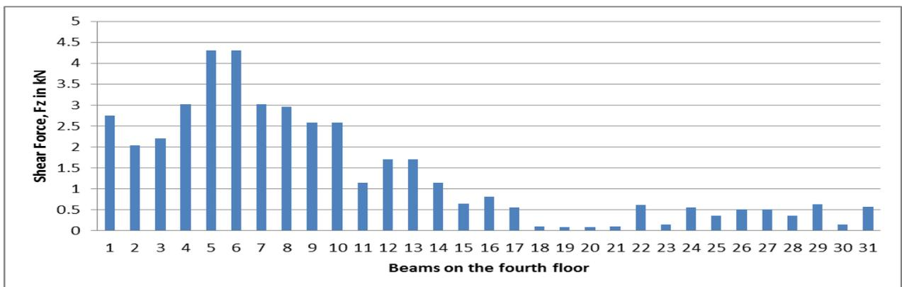
Graph-No. 6. Shear Force (Fz) for the beams on fourth floor
