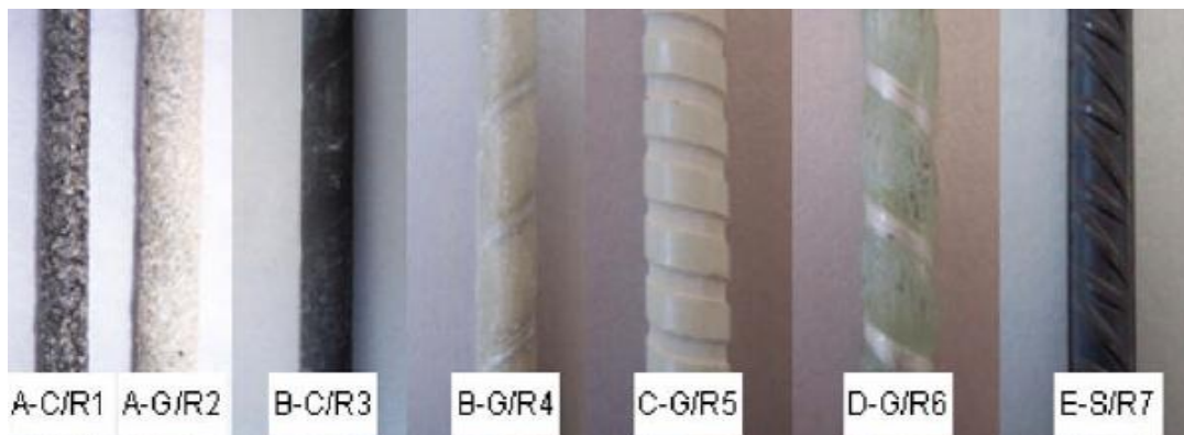
Figure-6. Surface deformations of FRP bars
