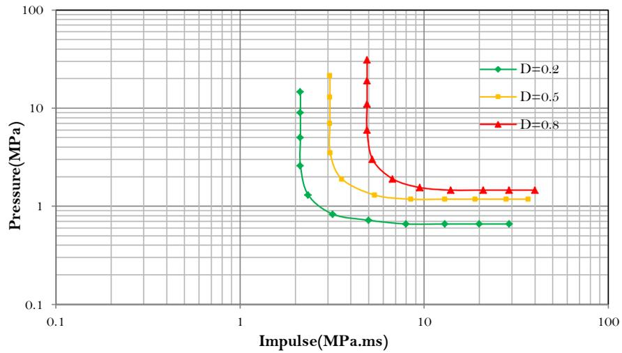
Figure-5. P-I diagram for RC column C2
