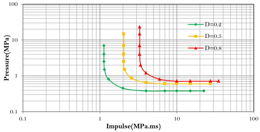
Figure-4. P-I diagram for RC column C1
