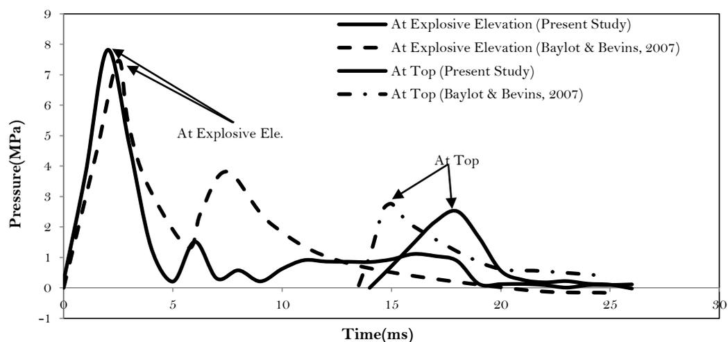
Figure-3. Pressure time histories for column in test No. 2 using ALE method
