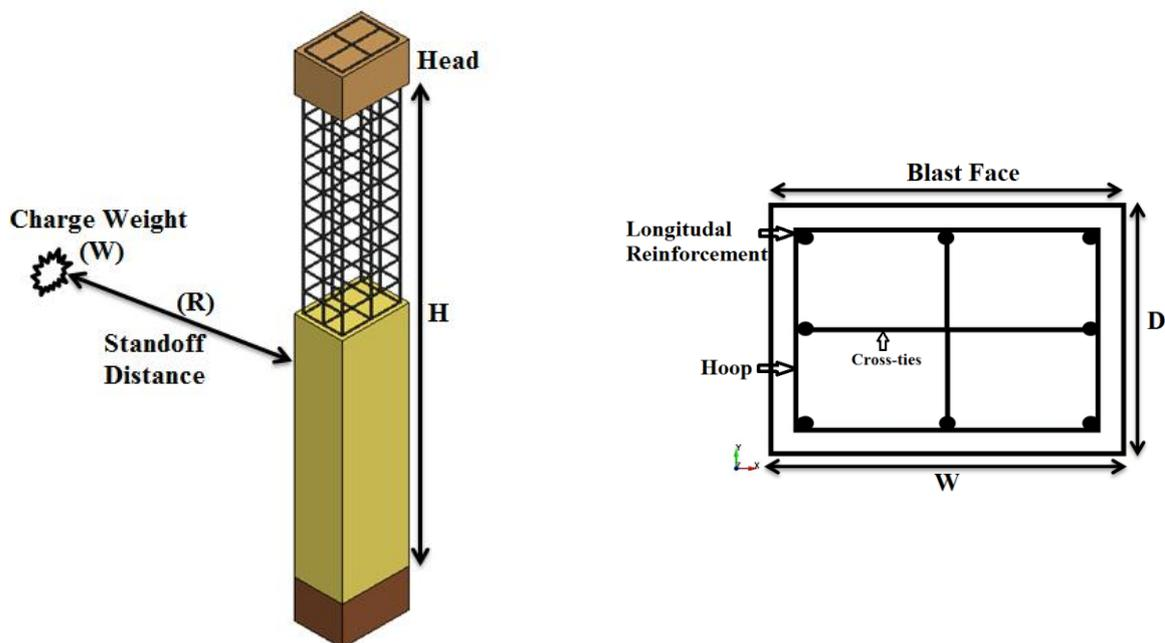
Figure-1. Details of RC column
