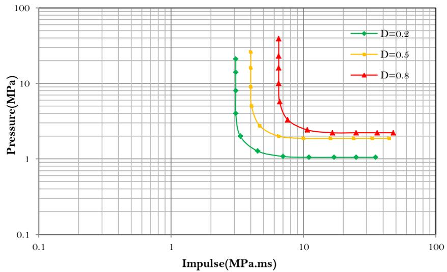
Figure-6. P-I diagram for RC column C3
