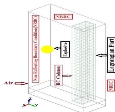
Figure-2. Numerical modelling of blast load
