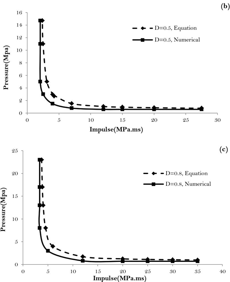
Figure-7. Comparison of P-I diagram for column C<sub>1</sub> generated from Eq. (4) and fitted numerical data.
