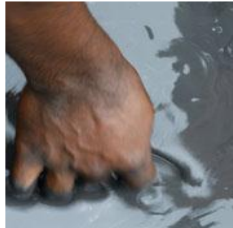
Figure-9. Coating in charcoal clay mixture.
