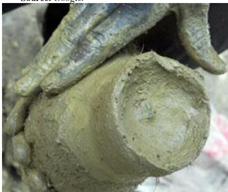
Figure-10. Coating with clay and palmfiber.
