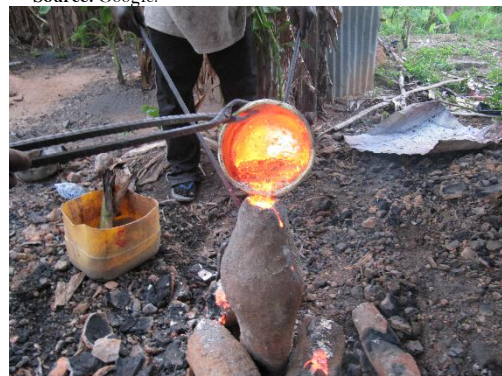
Figure-11. Casting process.
