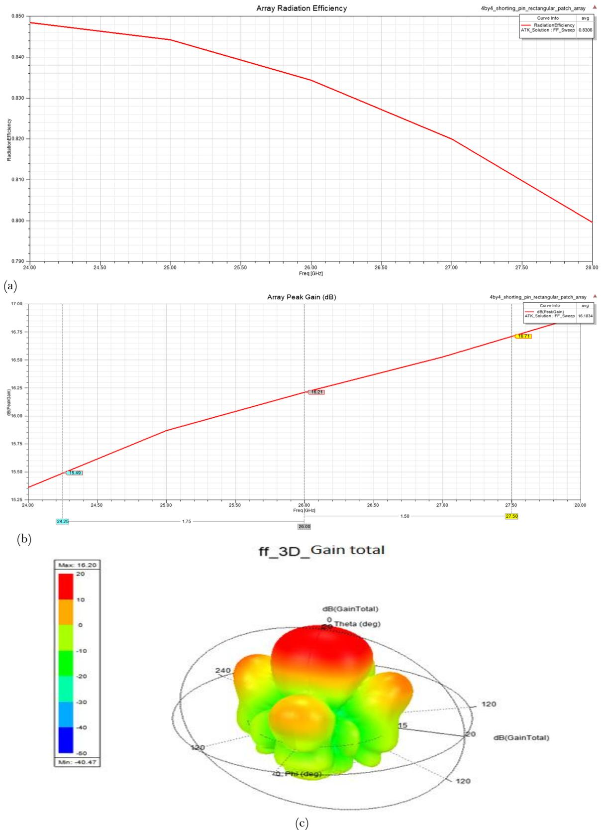
Figure-8. Antenna array results (a) Radiation efficiency (b) Antenna gain (c) 3D directivity plot.
