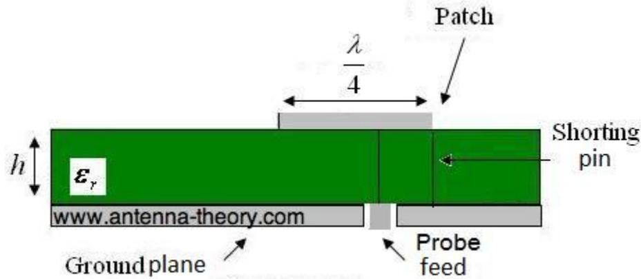
Figure-1. The planar inverted-F antenna (PIFA).
