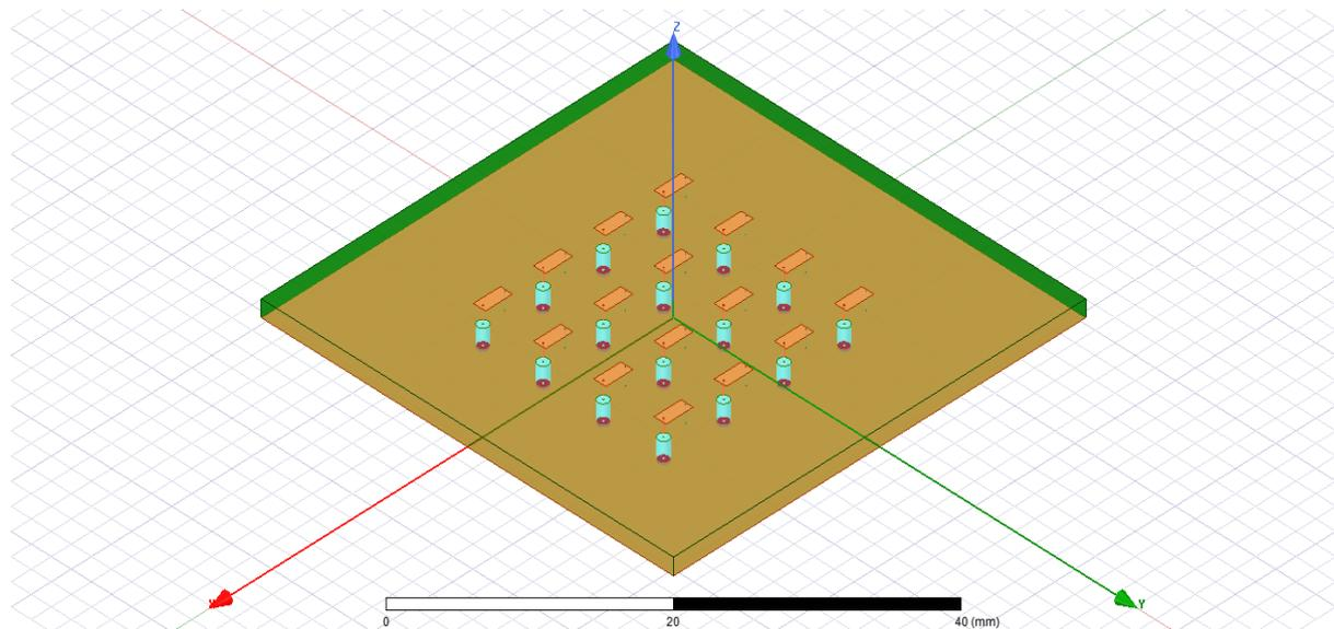
Figure-7. 16 element 4 x 4 antenna array design.
