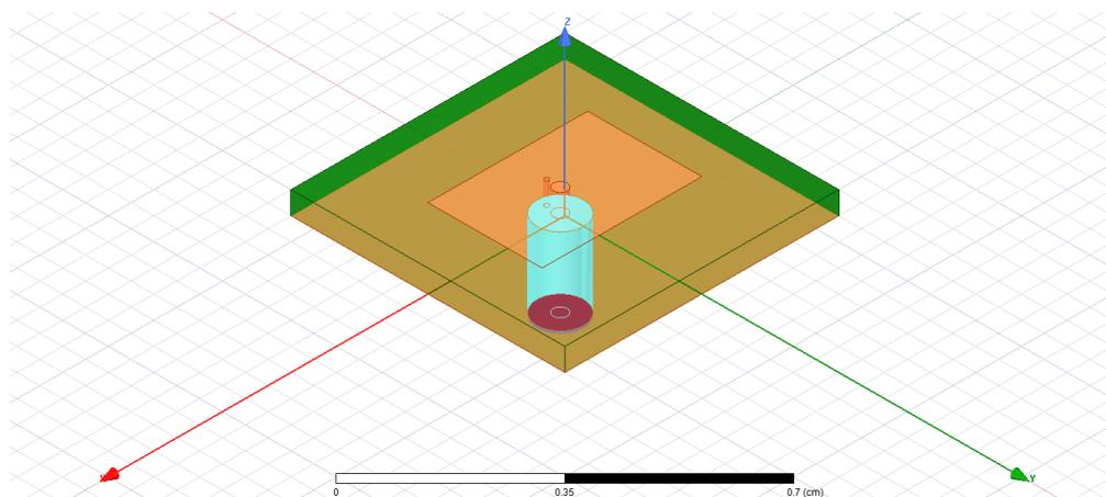
Figure-2. Proposed antenna design with substrate perspective view.
