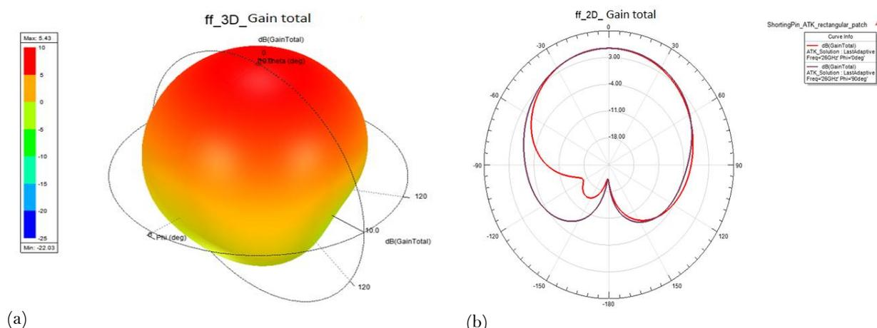
**Figure-3. Result (a) 3D directivity plot at 26 GHz (b) 2D polar plot.**
