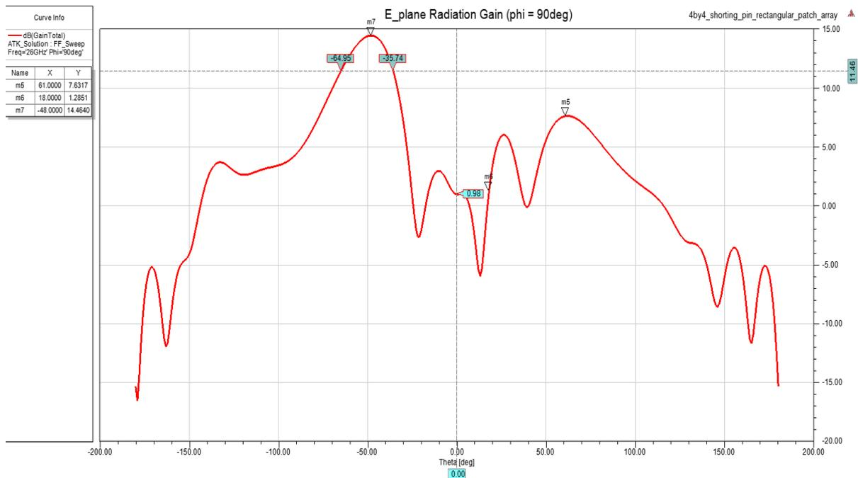
Figure-9. Radiation pattern for maximum scan angle.
