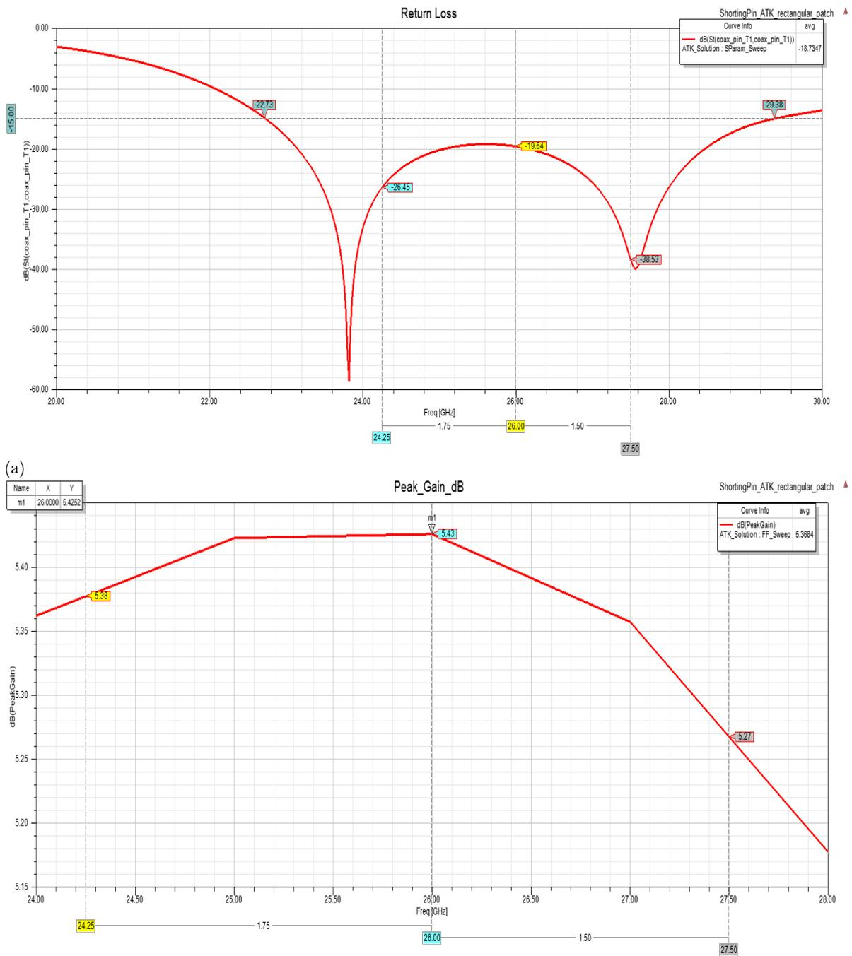
Figure-4. (a) Return Loss ( $S_{11}$  parameter) (b) Gain Plot (dB).
