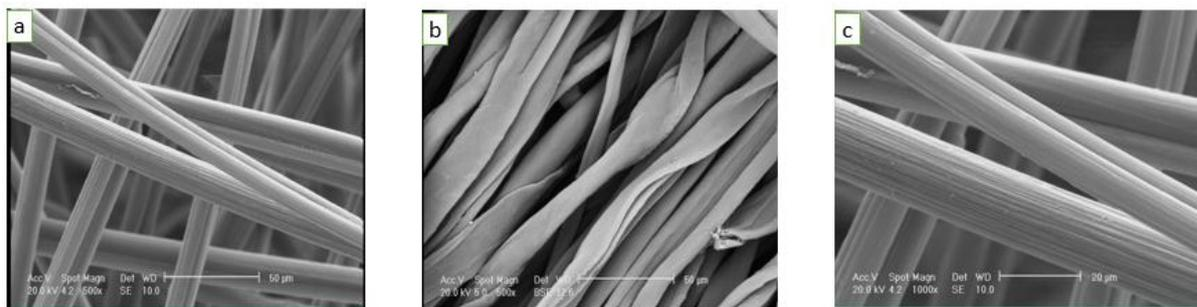
Figure-1. SEM of a. Calcium Alginate 20% / CMC , b. Calcium alginate 25% / CMC and c. Calcium alginate / CMC / propolis.
