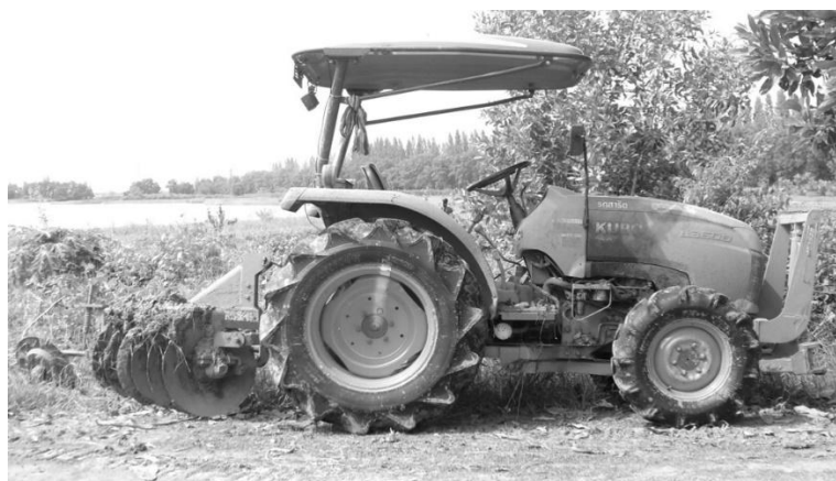
Figure 2. A 36-horsepower diesel wheeled tractor.
