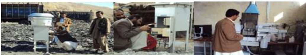
Figure-7. Collection and Analysis of coal dust sample in the field and EPA laboratory
