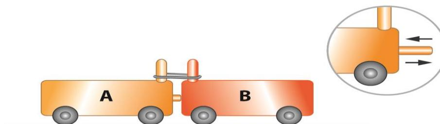
Figure-8. Visual effects of action and reaction pair of forces
